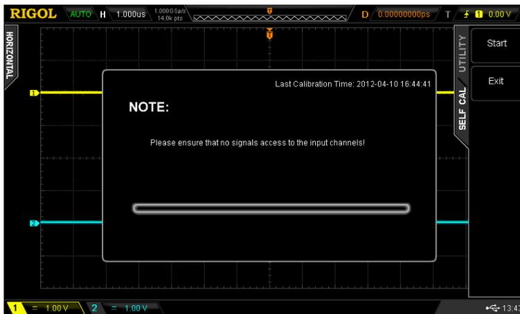
Press **Start** and the oscilloscope will start to execute the self-calibration program. Press **Exit** to give up the self-calibration operation at any time and return to the previous menu.
