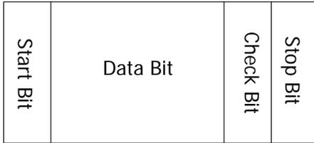
**Start Bit:** represent when the data starts outputting. Setting the **Polarity** is equivalent to specifying the "Start Bit".
