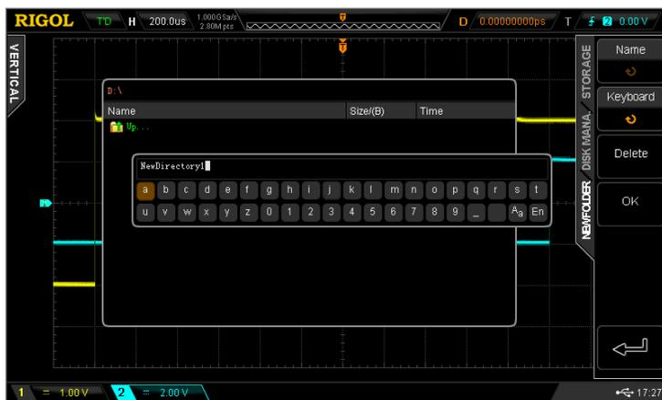
This oscilloscope supports Chinese/English input method. The file name or folder name can contain letters, numbers, underscores, spaces and Chinese characters and the length of the characters is limited to 64 bytes. The following part introduces how to input a file name or folder name using Chinese/English input method.
