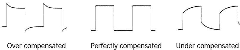
Figure 1-8 Probe Compensation
