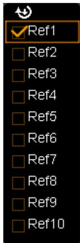
When the REF function is enabled, you can select different color for each reference waveform, set the source of each reference channel, adjust the vertical scale and position of the reference waveform and save the reference waveform to internal or external memory as well as recall it when needed. For details, please refer to the introductions below.
