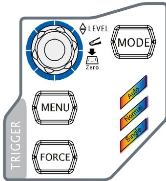
**MODE**: press this key to switch the trigger mode to **Auto**, **Normal** or **Single** and the corresponding state backlight of the current trigger mode would be illuminated.
