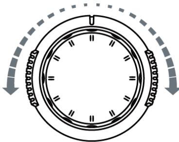
This knob provides quick Adjust/Locate function for numerical parameters with relatively larger settable range. Turn clockwise (counterclockwise) to increase (reduce) the value. The inner knob is used for fine adjustment and the outer knob for coarse adjustment.
