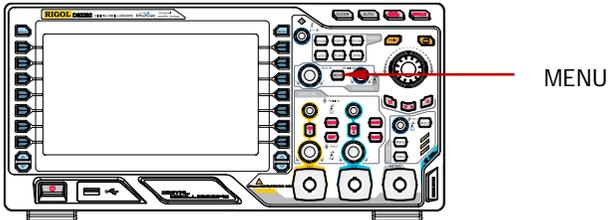
Press **MENU** in the horizontal control area (HORIZONTAL) at the front panel and press **Delayed** to enable or disable delayed sweep. Note that to enable delayed sweep, the current time base mode must be "Y-T" and the "Pass/Fail test" must be disabled.
