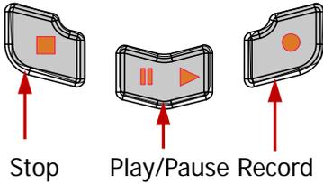
**Record:** press this key to start recording the waveform. The backlight is illuminated in red. Besides, when record constant on (Open) is enabled, the backlight will also be illuminated.
