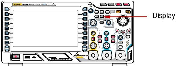
Press **Display** → **Type** to set the waveform display mode to “Vectors” or “Dots”.
