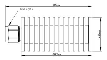
Coaxial fixed termination is used in absorbing energy of transmission line, expanding power range and controlling power level, they are also used in accurately measuring power or spectrum of RF microwave transmitters accompany with small power meter, comprehensive tester or spectrum analyzer.
