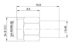
Coaxial fixed terminations absorb RF & microwave energy and are commonly used as dummy loads of antenna and transmitter. They are also used as match ports in many multiport microwave devices such as circulator and directional coupler to make these ports which are not involved in the measurement be terminated in their characteristic impedance in order to ensure an accurate measurement.
