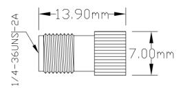
Coaxial fixed terminations absorb RF & microwave energy and are commonly used as dummy loads of antenna and transmitter. They are also used as match ports in many multiport microwave devices such as circulator and directional coupler to make these ports which are not involved in the measurement be terminated in their characteristic impedance in order to ensure an accurate measurement.
