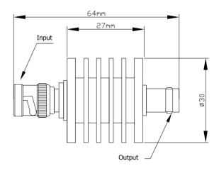
Coaxial fixed attenuators are used in absorbing energy of transmission line, expanding power range and controlling power level, they are also used in accurately measuring power or spectrum of RF microwave transmitters accompany with small power meter, comprehensive tester or spectrum analyzer.
