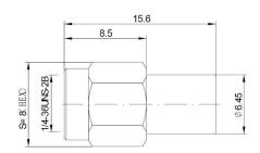
Coaxial fixed terminations absorb RF& microwave energy and are commonly used as dummy loads of antenna and transmitter. They are also used as match ports in many multiport microwave device such as circulator and directional coupler to make these ports which are not involved in the measurement be terminated in their characteristic impedance in order to ensure an accurate measurement.
