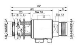
LA surge protectors look like in-line coaxial adapters using interfaces like N or 7/16, and that contain a field replaceable gas capsule placed between their inner and outer conductors. Unlike single band quarter wave protectors, gas tube surge arresters can be used for broadband applications. Their operating frequency band is DC to 6.0GHz.
