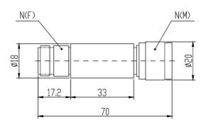
Coaxial fixed attenuators are used in absorbing energy of transmission line, expanding power range and controlling power level, they are also used in accurately measuring power or spectrum of RF microwave transmitters accompany with small power meter, comprehensive tester or spectrum analyzer.
