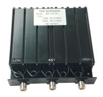
Compact duplexer 6MC450-50 is meant to provide frequency isolation between transmitting and receiving channels. Combining small geometry with low loss and close frequency spacing with selective pass characteristics this duplexer is ideal for use in systems with low-to-medium power repeaters where small physical dimensions of equipment are critical.
