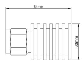
Coaxial fixed termination are used in absorbing energy of transmission line, expanding power range and controlling power level, they are also used in accurately measuring power or spectrum of RF microwave transmitters accompany with small power meter, comprehensive tester or spectrum analyzer.
