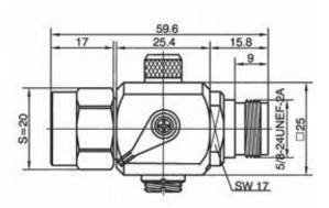
LA surge protectors look like in-line coaxial adapters using interfaces like N or 7/16, and that contain a field replaceable gas capsule placed between their inner and outer conductors. Unlike single band quarter wave protectors, gas tube surge arresters can be used for broadband applications. Their operating frequency band is DC to 3.5GHz.
