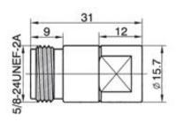
Coaxial fixed termination are used in absorbing energy of transmission line, expanding power range and controlling power level, they are also used in accurately measuring power or spectrum of RF microwave transmitters accompany with small power meter, comprehensive tester or spectrum analyzer.
