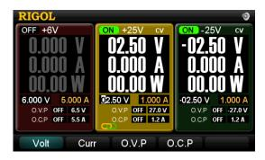
Figure 2-17 Tracking output (after tracking)
