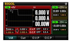
Figure 1-8 Focus waveform display mode
