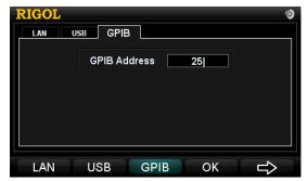
Figure 2-25 Set the GPIB address
