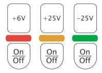
Figure 1-4 Output channel selection
