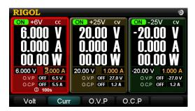
Figure 2-13 Timing output (normal display mode)
