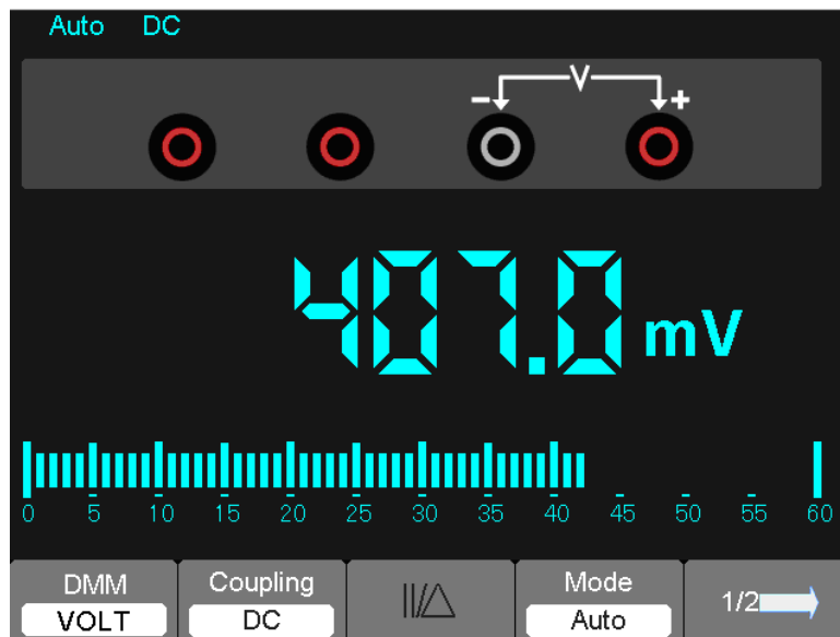
Figure 7-6 DC voltage Measurement
