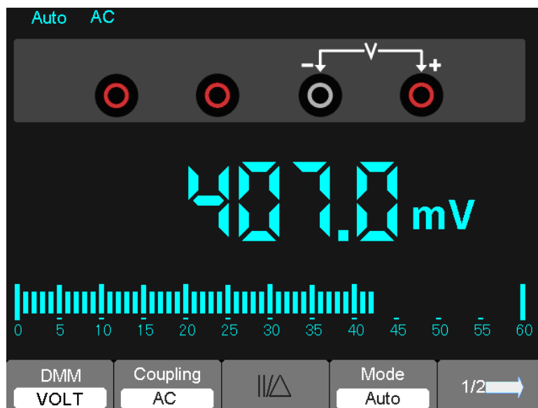
Figure 7-7 AC voltage Measurement
